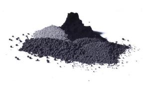
Figure 1a: Representative picture of Carbon Black as typically placed on the market
